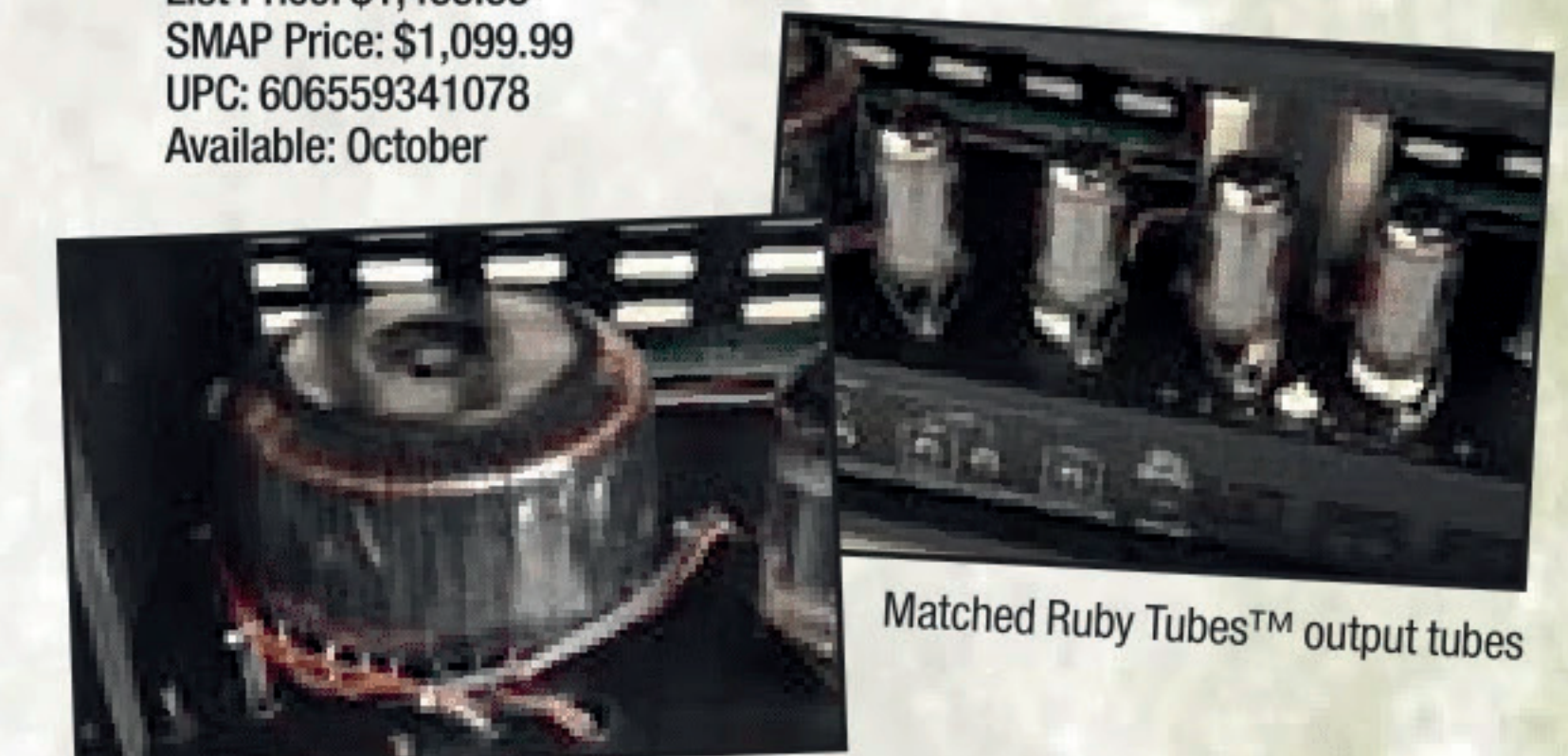
High efficiency toroidal core transformer
