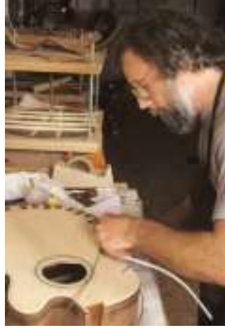
▲ Mike Bakeberg applies binding on a Custom cutaway.
