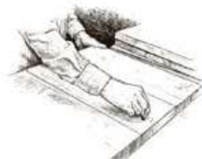
Matching wood panels for grain and color
