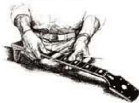
Fret board positioning and installation
