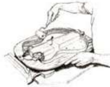
Hand application of top & bottom to rims
