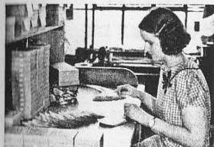
Individual inspection awaits every Gibson string. It is coiled by hand, put into a strong glassine envelope and then packed in the famous orange and black box.
