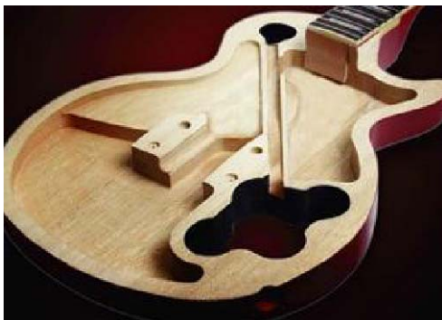
Computer designed body cavities for a more "acoustic" tone
