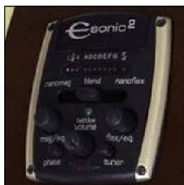
The eSonic-2™ stereo preamp with built-in tuner, stereo outputs, and NanoMag™ EQ
