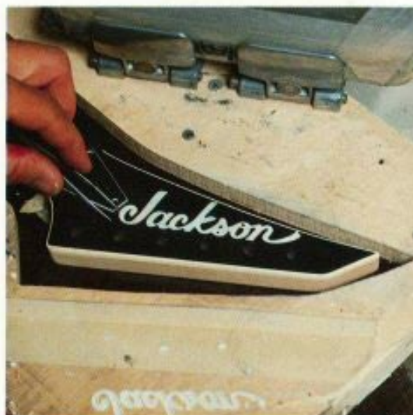
Logo Application. Logos are applied by silk-screen or decal. A pearl logo is being hand-placed in this photo.
