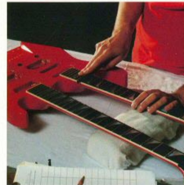
Neck/Fret Dress. The ultimate playing surface on a guitar is the frets. There are no machines in this department. All fretwork is done by hand to insure that the guitar plays flawlessly.
