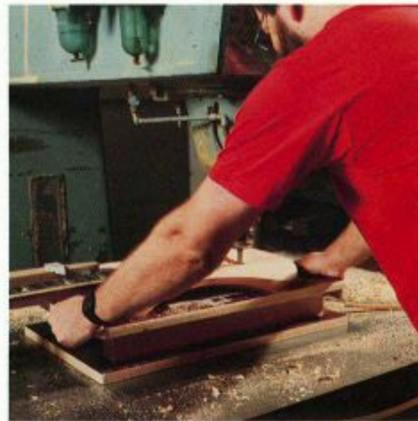
Shaping/Cavity Routing. All Jackson guitar bodies are hand routed using custom hand-made jigs to insure proper tolerances and specifications.
