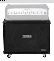
The 115 PRO cabinet delivers the big, warm sound that only a 15" speaker can deliver. Features include a cast-frame Fender® Special Design Eminence® 15" driver, compression driver horn with attenuator, carpet covering, stacking corners, a metal grille, removable casters, Speakon® and 1/4" jacks and banana plugs. Rated at 700 watts program (350 watts continuous at 8 ohms).
