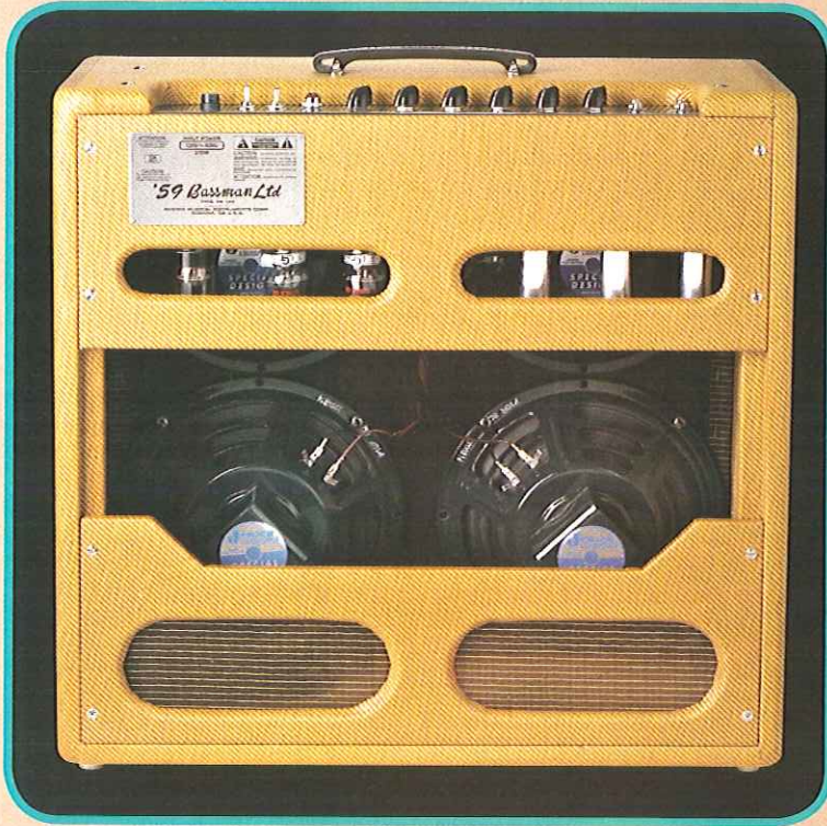
The '59 Bassman® LTD is loaded with four 10" 8 Ohm Jensen P10R speakers with Alnico magnets.
