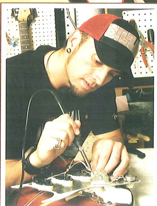
Artist Relations Manager and Custom Shop veteran, Alex Perez, installs some pickups on a Stratocaster® guitar.
