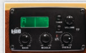
B-Band Electronics w/ 3-band EQ and digital tuner
