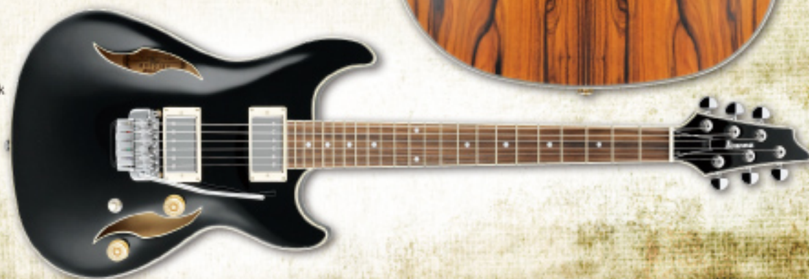
ACT Tremolo The first knife-edge tremolo designed for semi-acoustic guitar, the ACT eliminates the tremolo cavity that sacrifices the tone. Shorter springs use less vibrating room and contribute to a stiffer arm response. Two ways to install the springs offer choice in string and arm tension. And on top of all that, the ACT is smooth to the touch and string changes are easy.
