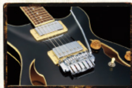
ACT Tremolo The first knife-edge tremolo designed for semi-acoustic guitar, the ACT eliminates the tremolo cavity that sacrifices the tone. Shorter springs use less vibrating room and contribute to a stiffer arm response. Two ways to install the springs offer choice in string and arm tension. And on top of all that, the ACT is smooth to the touch and string changes are easy.
