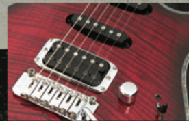
True Duo humbucker. Original Ibanez design (Patent pending) triple-coil construction (one single with one stacked) makes Ibanez the first to achieve switching between genuine single-coil and humbucking tone in one pickup.
