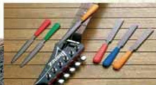
4451 (left) Nut File Set (3pcs. =1set) file gauge (inch): 0.012 & 0.032/0.016 & 0.042/0.025 & 0.052 4450 (right) Fret File Set (3pcs. =1set) file gauge (inch): 0.079, 0.098, 0.118
