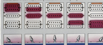
Position 1: Neck pickup Position 2: Neck (bridge side coil only) and Middle Position 3: Middle pickup Position 4: Middle and Bridge (lead side coil only) Position 5: Bridge pickup
